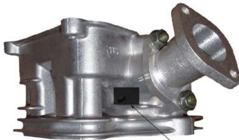
Approved Yamaha YF200 Inlet Tract Repair Area
